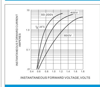
Fig.1 FORWARD CHARACTERISTICS
