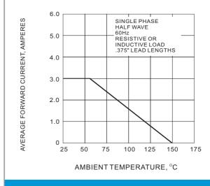
Fig.2 FORWARD CURRENT DERATING CURVE
