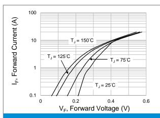
**Fig.4 Typical Forward Characteristics**
