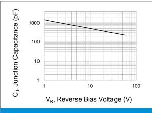
Fig.2 Typical Junction Capacitance
