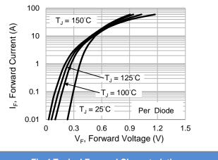
Fig.4 Typical Forward Characteristics
