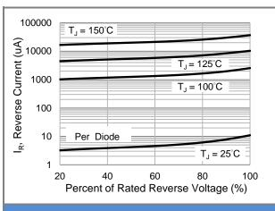
Fig.3 Typical Reverse Characteristics
