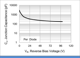
Fig.2 Typical Junction Capacitance
