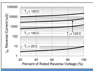
Fig.3 Typical Reverse Characteristics
