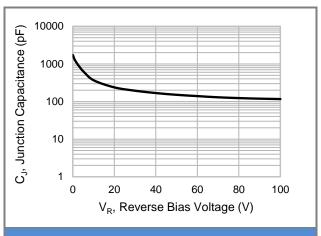
**Fig.2 Typical Junction Capacitance**
