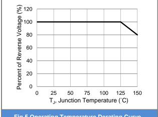
Fig.5 Operating Temperature Derating Curve
