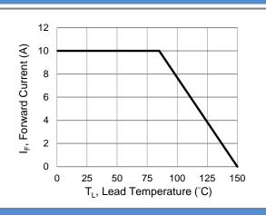
Fig.1 Forward Current Derating Curve
