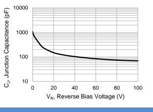
Fig.2 Typical Junction Capacitance
