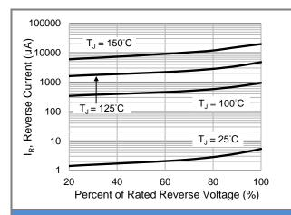
**Fig.3 Typical Reverse Characteristics**
