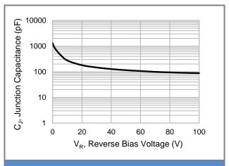
Fig.2 Typical Junction Capacitance
