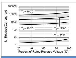
Fig.3 Typical Reverse Characteristics
