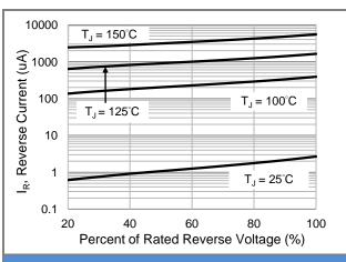
Fig.3 Typical Reverse Characteristics
