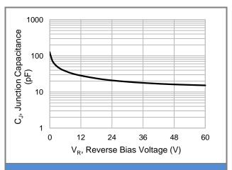
**Fig.2 Typical Junction Capacitance**
