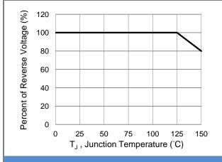
Fig.5 Operating Temperature Derating Curve
