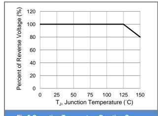
Fig.5 Operating Temperature Derating Curve
