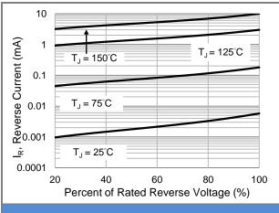
Fig.3 Typical Reverse Characteristics
