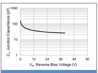
**Fig.2 Typical Junction Capacitance**
