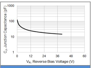
**Fig.2 Typical Junction Capacitance**
