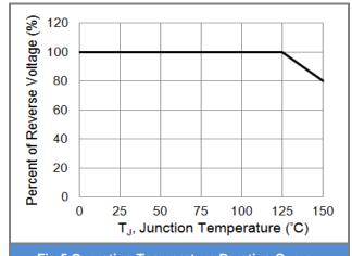
Fig.5 Operating Temperature Derating Curve
