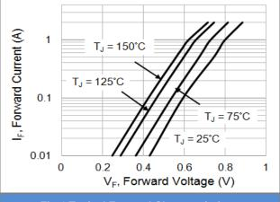
Fig.4 Typical Forward Characteristics
