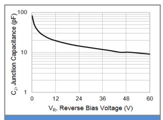
**Fig.2 Typical Junction Capacitance**
