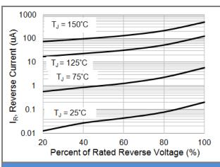
Fig.3 Typical Reverse Characteristics
