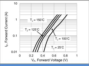
Fig.4 Typical Forward Characteristics
