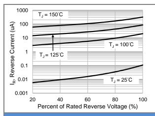
Fig.3 Typical Reverse Characteristics
