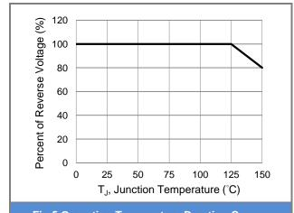
Fig.5 Operating Temperature Derating Curve
