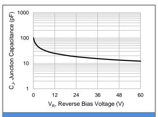
**Fig.2 Typical Junction Capacitance**
