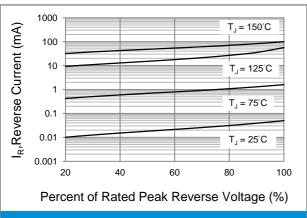
Fig.3 Typical Reverse Characteristics
