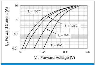
Fig.4 Typical Forward Characteristics
