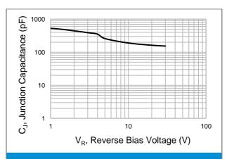
**Fig.2 Typical Junction Capacitance**
