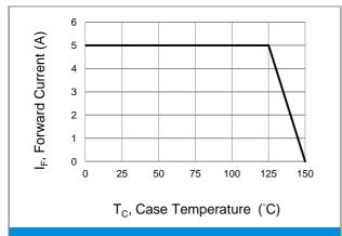
**Fig.1 Forward Current Derating Curve**
