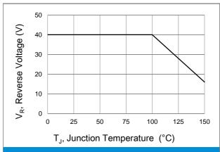
**Fig.5 Operating Temperature Derating Curve**
