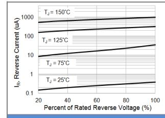
Fig.3 Typical Reverse Characteristics
