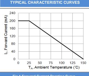
Fig.1 Forward Current Derating Curve
