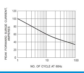
Fig.4 MAXIMUM NON-REPETITIVEPEAK FORWARD SURGE CURRENT
