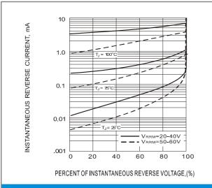
Fig.3 TYPICAL REVERSE CHARACTERISTICS
