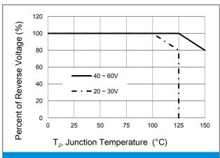
Fig.5 Operating Temperature Derating Curve
