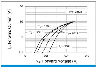
**Fig.4 Typical Forward Characteristics**
