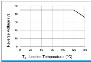
Fig.5 Operating Temperature Derating Curve
