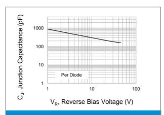
Fig.2 Typical Junction Capacitance
