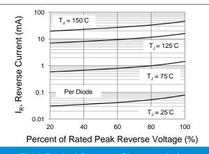
Fig.3 Typical Reverse Characteristics
