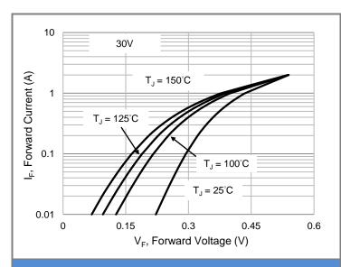
Fig.7 Typical Forward Characteristics
