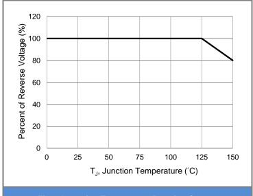
**Fig.9 Operating Temperature Derating Curve**
