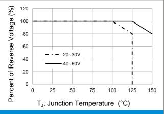
Fig.5 Operating Temperature Derating Curve
