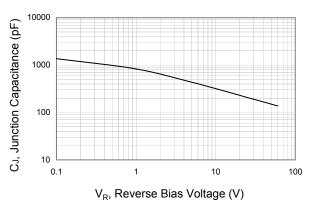
Fig.4 Typical Junction Capacitance under Bias
