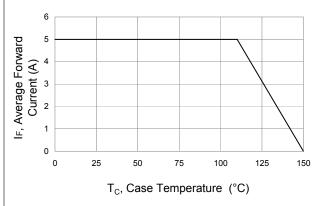
Fig.3 Forward Current Derating Curve
