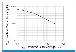
**Fig.2 Typical Junction Capacitance**
