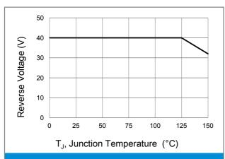
**Fig.5 Operating Temperature Derating Curve**
