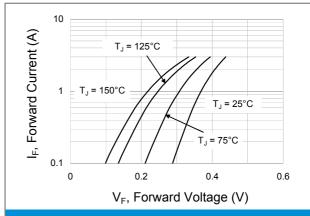
**Fig.4 Typical Forward Characteristics**
