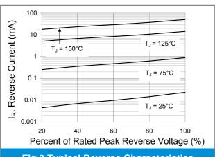
Fig.3 Typical Reverse Characteristics
