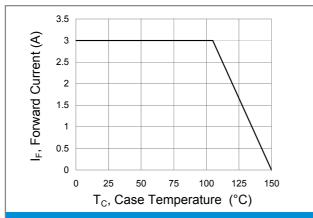
**Fig.1 Forward Current Derating Curve**
