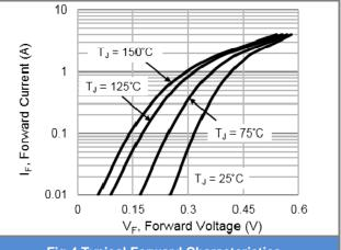
Fig.4 Typical Forward Characteristics
