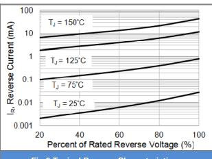
**Fig.3 Typical Reverse Characteristics**
