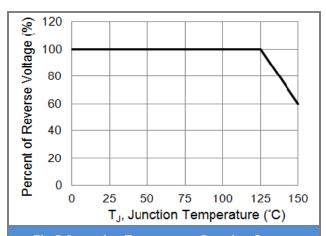
**Fig.5 Operating Temperature Derating Curve**
