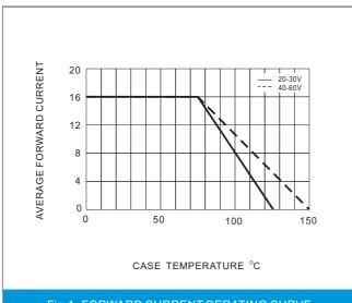
Fig.1- FORWARD CURRENT DERATING CURVE
