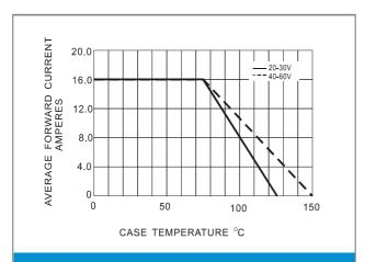
Fig.1- FORWARD CURRENT DERATING CURVE
