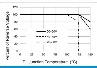
**Fig.5 Operating Temperature Derating Curve**
