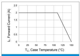
**Fig.1 Forward Current Derating Curve**
