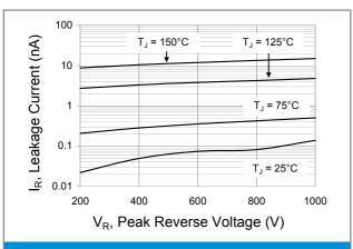
Fig.3 Typical Reverse Characteristics
