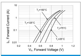
**Fig.4 Typical Forward Characteristics**
