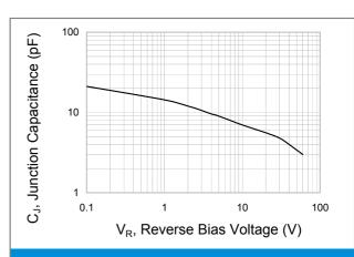
**Fig.2 Typical Junction Capacitance**
