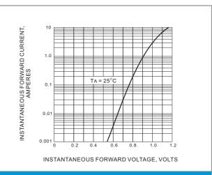
FIG.2 TYPICAL FORWARD CHARACTERISTICS
