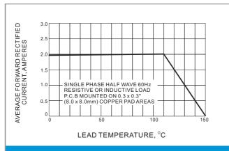
Fig.1 FORWARD CURRENT DERATING CURVE
