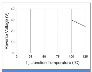
**Fig.1 Operating Temperature Derating Curve**
