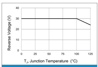
Fig.6 Operating Temperature Derating Curve
