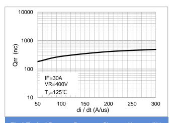
Fig.6 Typical Reverse Recovery Charges Versus di/dt
