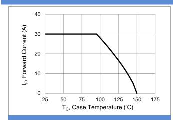
**Fig.1 Forward Current Derating Curve**
