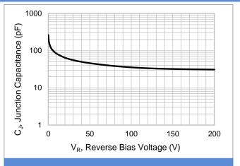
Fig.2 Typical Junction Capacitance
