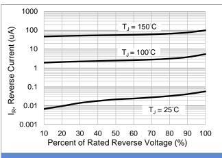
Fig.3 Typical Reverse Characteristics
