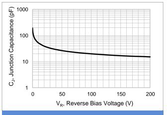
Fig.2 Typical Junction Capacitance
