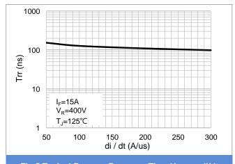
Fig.5 Typical Reverse Recovery Time Versus di/dt
