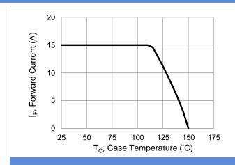
**Fig.1 Forward Current Derating Curve**
