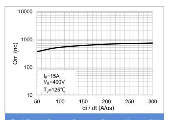
Fig.6 Typical Reverse Recovery Charges Versus di/dt
