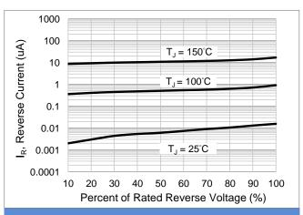
Fig.3 Typical Reverse Characteristics
