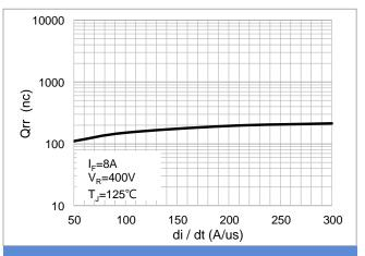
Fig.6 Typical Reverse Recovery Charges Versus di/dt
