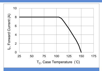
**Fig.1 Forward Current Derating Curve**
