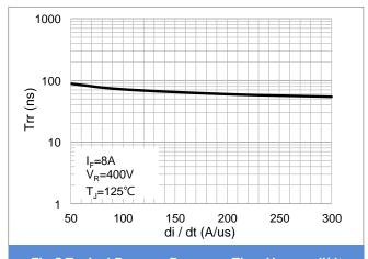
Fig.5 Typical Reverse Recovery Time Versus di/dt
