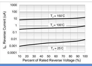
**Fig.3 Typical Reverse Characteristics**
