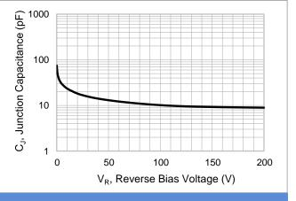
Fig.2 Typical Junction Capacitance
