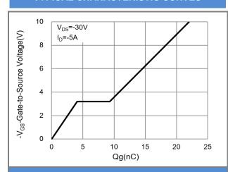
Fig.7 Gate-Charge Characteristics
