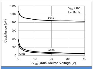
Fig.10 Capacitance vs. Drain-Source Voltage
