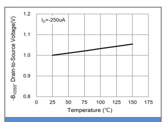
Fig.8 Breakdown Voltage Variation vs. Temperature
