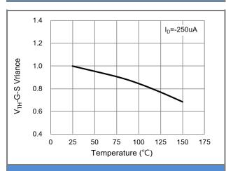
Fig.9 Threshold Voltage Variation with Temperature
