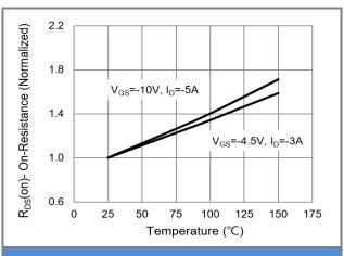
Fig.4 On-Resistance vs. Junction temperature
