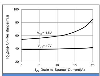
Fig.3 On-Resistance vs. Drain Current
