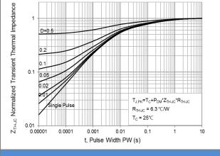
Fig.12 Normalized Transient Thermal Impedance
