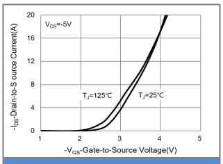
Fig.2 Transfer Characteristics
