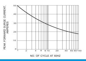
Fig.2- MAXIMUM OVERLOAD SURGE CURRENT
