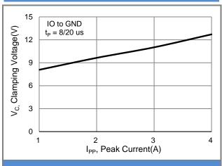
Fig.1 Typical Peak Clamping Voltage
