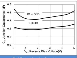
Fig.3 Typical Junction Capacitance
