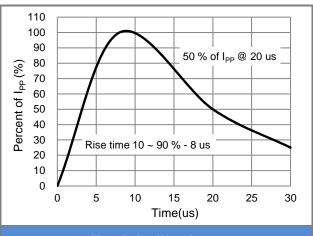
Fig.2 Pulse Waveform
