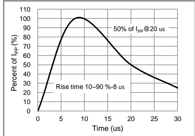
Fig.2 Pulse Waveform
