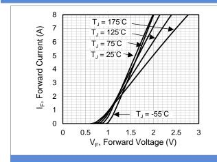
**Fig.1 Forward Characteristics**
