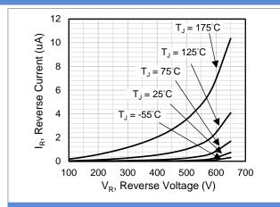
Fig.2 Reverse Characteristics
