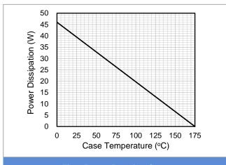
**Fig.3 Power Derating Curve**
