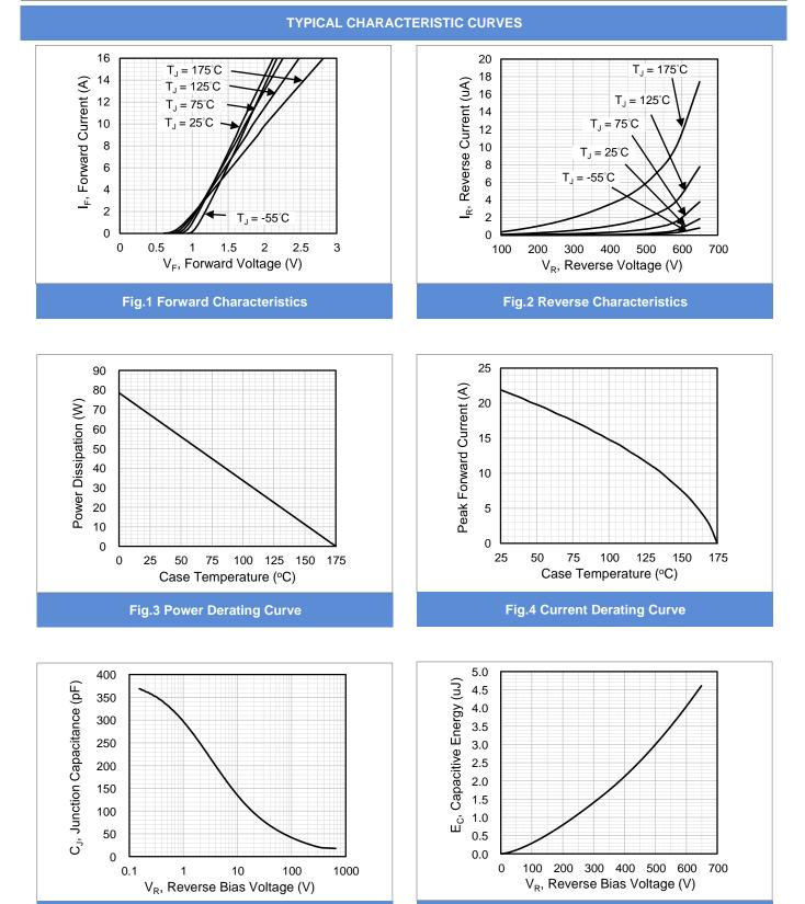
**Fig.5 Typical Junction Capacitance**
