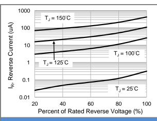
Fig.3 Typical Reverse Characteristics
