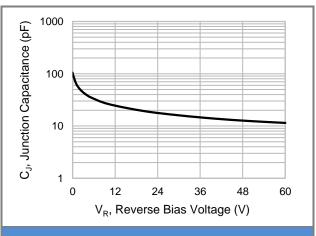
**Fig.2 Typical Junction Capacitance**
