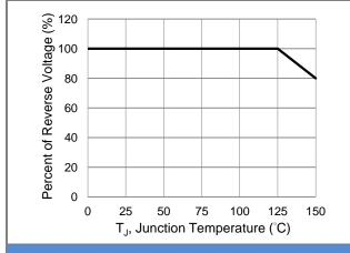
Fig.5 Operating Temperature Derating Curve
