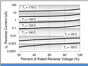
Fig.3 Typical Reverse Characteristics
