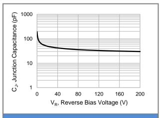
Fig.2 Typical Junction Capacitance
