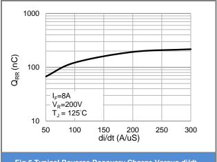
Fig.6 Typical Reverse Recovery Charge Versus di/dt
