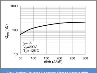
Fig.6 Typical Reverse Recovery Charge Versus di/dt
