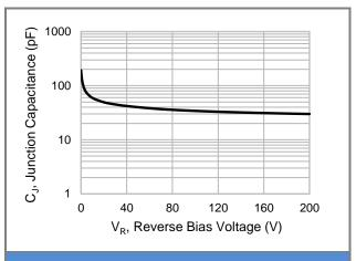
Fig.2 Typical Junction Capacitance
