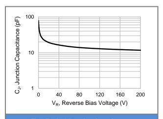
Fig.2 Typical Junction Capacitance
