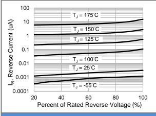
Fig.3 Typical Reverse Characteristics
