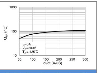
Fig.6 Typical Reverse Recovery Charge Versus di/dt
