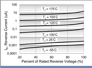
Fig.3 Typical Reverse Characteristics
