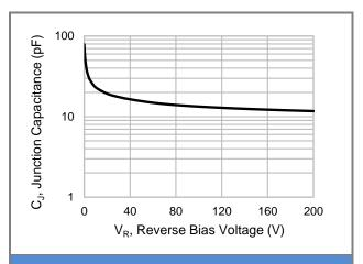
Fig.2 Typical Junction Capacitance
