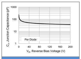
Fig.2 Typical Junction Capacitance
