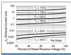
Fig.3 Typical Reverse Characteristics
