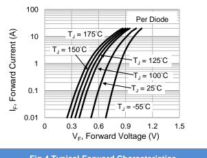
Fig.4 Typical Forward Characteristics
