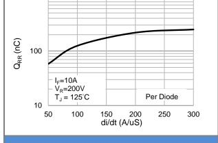
Fig.6 Typical Reverse Recovery Charge Versus di/dt
