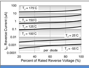
Fig.3 Typical Reverse Characteristics
