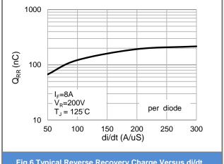
Fig.6 Typical Reverse Recovery Charge Versus di/dt
