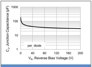
Fig.2 Typical Junction Capacitance
