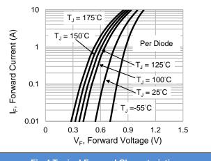
Fig.4 Typical Forward Characteristics
