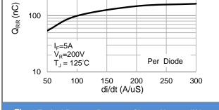
Fig. 6 Typical Reverse Recovery Charge Versus di/dt
