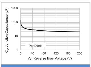
Fig.2 Typical Junction Capacitance
