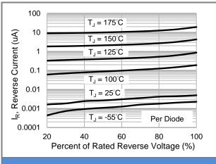
Fig.3 Typical Reverse Characteristics
