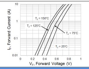
Fig.4 Typical Forward Characteristics
