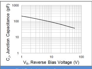
Fig.2 Typical Junction Capacitance
