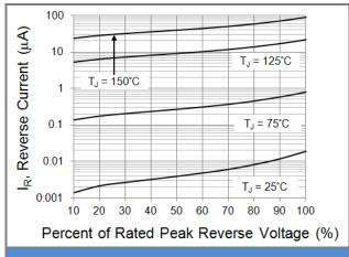
Fig.3 Typical Reverse Characteristics
