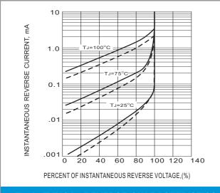
Fig.3- TYPICAL REVERSE CHARACTERISTICS
