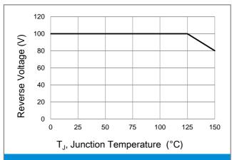
Fig.5 Operating Temperature Derating Curve
