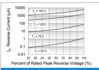
Fig.3 Typical Reverse Characteristics
