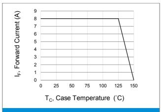
**Fig.1 Forward Current Derating Curve**
