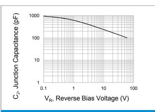
**Fig.2 Typical Junction Capacitance**
