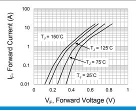
Fig.4 Typical Forward Characteristics
