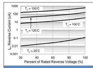
Fig.3 Typical Reverse Characteristics
