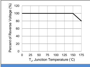
Fig.5 Operating Temperature Derating Curve
