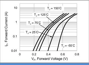
Fig.4 Typical Forward Characteristics
