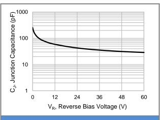
**Fig.2 Typical Junction Capacitance**
