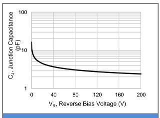
**Fig.2 Typical Junction Capacitance**
