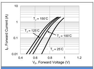
Fig.4 Typical Forward Characteristics
