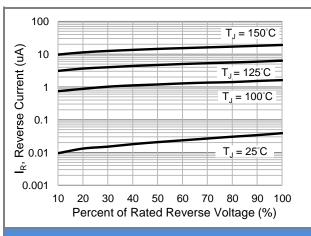
Fig.3 Typical Reverse Characteristics
