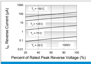
Fig.4 Typical Reverse Characteristics
