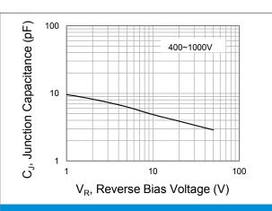
**Fig.2 Typical Junction Capacitance**
