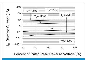
Fig.3 Typical Reverse Characteristics
