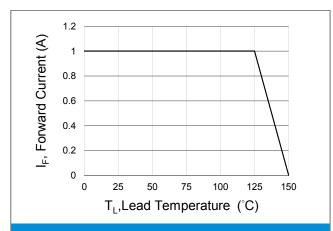
**Fig.1 Forward Current Derating Curve**
